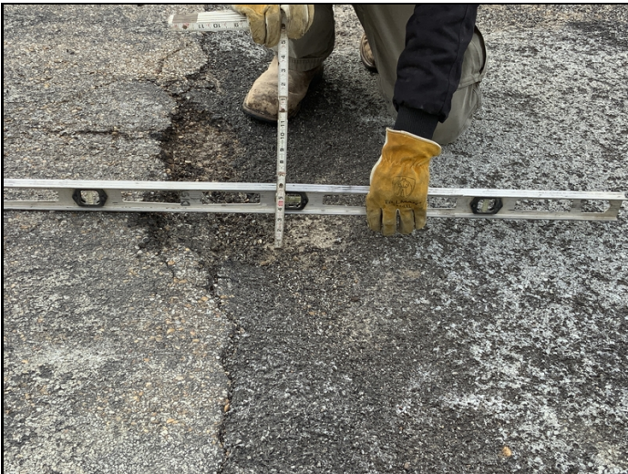
Abutment #2 approach roadway settlement.
